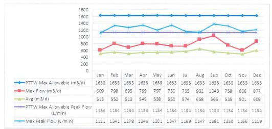
The above table shows there were spikes in <u>instantaneous</u> peak flow rate (L/min) and max flow rate these occurrences were caused during pump start-up/pump to waste. The Peak Flow rate increased in September 2022 during Well #3 Pump maintenance after a failure.
