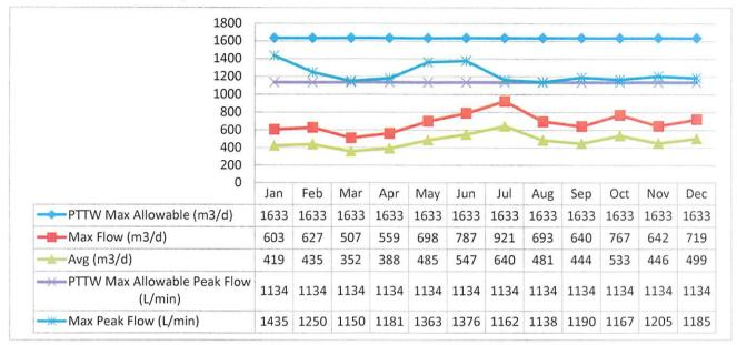
The above table shows there were spikes in <u>instantaneous</u> peak flow rate (L/min) and max flow rate these occurrences were caused during pump start-up/pump to waste. The Peak Flow rate was increased in May 2020 during scheduled flow meter calibrations.
